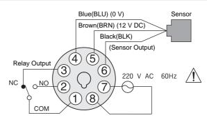
The controller (HPA-12) for sensor has the output circuit which operates the power relay as amplifying the output of NPN type and PNP type and the power circuit for sensor. If the sensor detects an object, the relay will be operating.
